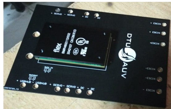
Power distribution board
